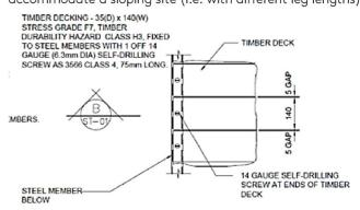
The platform must be in direct contact with minimum 95% of the area of the base of the tank and large enough to support all edges of the tank. With reference to the picture above, the recommended gap between the timber decking boards is 5 mm and must never be greater than 25mm. The tank stand must be level with no more than a 1°slope.
